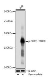
Western blot analysis of extracts of Raji cells, using Phospho-SHIP1-Y1020 antibody (TA377517) at 1:1000 dilution.Raji cells were treated by Pervanadate (1 mM) at 37°C for 30 minutes. | Secondary antibody: HRP Goat Anti-Rabbit IgG (H+L) at 1:10000 dilution. | Lysates/proteins: 25ug per lane. | Blocking buffer: 3% nonfat dry milk in TBST. | Detection: ECL Basic Kit. | Exposure time: 1s.
