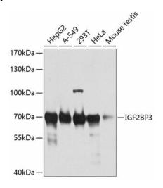
Western blot analysis of extracts of various cell lines, using IGF2BP3 antibody (TA377381) at 1:1000 dilution.|Secondary antibody: HRP Goat Anti-Rabbit IgG (H+L) at 1:10000 dilution.|Lysates/proteins: 25ug per lane.|Blocking buffer: 3% nonfat dry milk in TBST.|Detection: ECL Basic Kit.|Exposure time: 15s.
