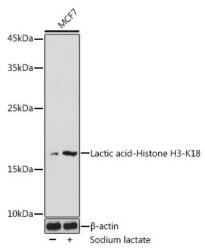
Western blot analysis of extracts of MCF7 cells, using Lactic acid-Histone H3-K18 antibody ([TA376901]) at 1:500 dilution.MCF7 cells were treated by Sodium lactate(100mM) for 24h. |Secondary antibody: HRP Goat Anti-Rabbit IgG (H+L) at 1:10000 dilution. |Lysates/proteins: 25ug per lane. |Blocking buffer: 3% BSA. |Detection: ECL Basic Kit. |Exposure time: 5min.
