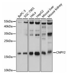
Western blot analysis of extracts of various cell lines, using CNPY2 antibody (TA374930) at 1:1000 dilution. | Secondary antibody: HRP Goat Anti-Rabbit IgG (H+L) at 1:10000 dilution. | Lysates/proteins: 25ug per lane. | Blocking buffer: 3% nonfat dry milk in TBST. | Detection: ECL Basic Kit. | Exposure time: 5s.
