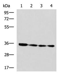
Gel: 8%SDS-PAGE Lysate: 40 µg Lane 1-4: 231 cell Jurkat cell PC3 and 293T cell lysates Primary antibody: [TA373010] (NUDT22 Antibody) at dilution 1/1300 Secondary antibody: Goat anti rabbit IgG at 1/5000 dilution
