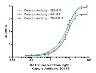
Standard Curve for H-FABP: Capture Antibody Mouse mAb (5C4-F5) to H-FABP at 4ug/ml and Detector Antibody Mouse mAb (3E8-B10, 7B10-G11, 4H1-B8)to H-FABP at 0.08 ug/ml.
