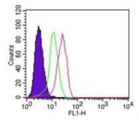
Flow Cytometry: IkB-alpha Antibody (6A920) TA336372 - Intracellular staining of 10^6 ThP-1 cells using 0.25 ug of TA336372. Shaded histogram represents cells alone, green represents the isotype control, and red represents the IkBa antibody. Novus's intracellular flow kit was used for this test, and an anti-mouse IgG FITC conjugated secondary.
