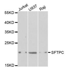
Western blot analysis of extracts of various cell lines, using SFTPC antibody.
