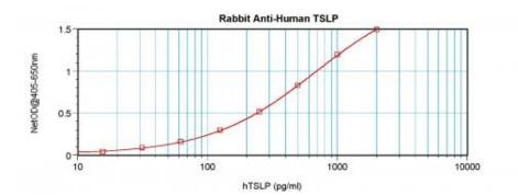
To detect hTSLP by sandwich ELISA (using 100 ul/well antibody solution) a concentration of 0.5 - 2.0 ug/ml of this antibody is required. This antigen affinity purified antibody, in conjunction with Biotinylated Anti-Human TSLP as a detection antibody, allows the detection of at least 0.2 - 0.4 ng/well of recombinant hTSLP.
