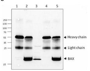
Immunoprecipitation/Western blot analysis of extracts from Daudi cells (lane 1 and lane 2) and THP-1 cells (lane 4 and Lane 5). Lane 4 contains THP-1 lysate input (5%). Lane 1 and lane 4 were immunoprecipitated with mouse IgG1 isotype control antibodies and lane 2 and lane 5 were immunoprecipitated with BAX antibody (6A7). Western blot analysis was performed using rabbit anti-BAX antibody (poly6251).
