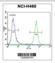
PURB Antibody (C-term) (Cat. #[TA324468]) flow cytometric analysis of NCI-H460 cells (right histogram) compared to a negative control cell (left histogram).FITC-conjugated goat-anti-rabbit secondary antibodies were used for the analysis.
