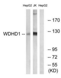
Western blot analysis of extracts from HepG2 cells and Jurkat cells, using WDHD1 antibody. The lane on the right is treated with the synthesized peptide.
