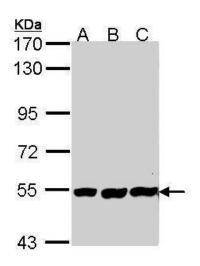
Sample (30 ug of whole cell lysate). A: H1299. B: Hela. C: Hep G2. 7.5% SDS PAGE. TA308470 diluted at 1:500.
