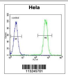
MAPK14 Antibody (Y323) (Cat. #TA302203) flow cytometric analysis of Hela cells (right histogram) compared to a negative control cell (left histogram).FITC-conjugated goat-anti-rabbit secondary antibodies were used for the analysis.
