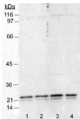
Western Blot: Caveolin-1 Antibody (7C8) TA301445 - Detection of caveolin in 3T3 cell lysates (50 ug). Lanes 1 and 2: 1:4000. Lanes 3 and 4: 1:1000. Detection by ECL: 5 minute exposure.
