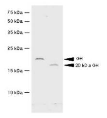
Immunoblot analysis: Recombinant hGH and 20kDa hGH were resolved by electrophoresis, transferred to PVDF membrane and probed with anti-Human GH antibody (1/500). Proteins were visualized using a goat anti-mouse secondary antibody conjugated to HRP and a DAB detection system. Arrows indicate recombinant hGH (22 kDa) and 20 kDa hGH, respectively.
