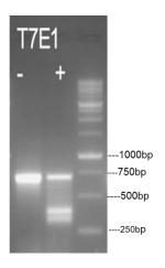
sgRNA targeting EMX1 gene was transduced into SK-BR-3/ Cas9-hyg Stable Cell Line by transduction. EMX1 gene was cut by CAS9 expressed inside the cells and repaired through NHEJ with mutation. A 684 bp EMX1 gene fragment from PCR was then tested by T7 Endonuclease I (T7 E1) Assay. The T7 E1 cleavage will result in two additional bands:
