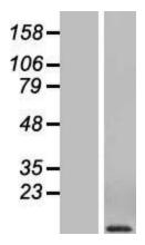
Western blot validation of overexpression lysate (Cat# [LY418970]) using anti-DDK antibody (Cat# [TA50011-100]). Left: Cell lysates from untransfected HEK293T cells; Right: Cell lysates from HEK293T cells transfected with RC210026 using transfection reagent MegaTran 2.0 (Cat# [TT210002]).
