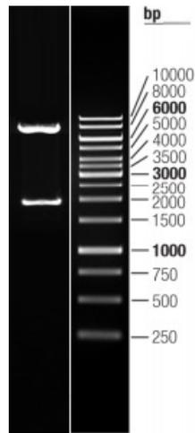
Double digestion of RC203447L4 using SgfI and MluI
