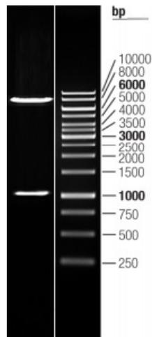
Double digestion of RC203032L4 using SgfI and MluI
