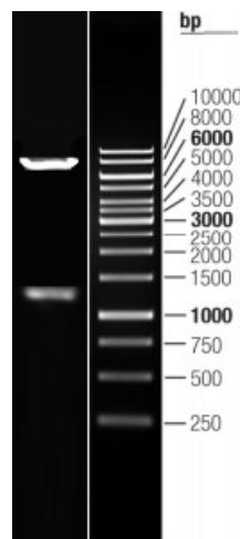
Double digestion of MR223037L4 using SgfI and RsrII
