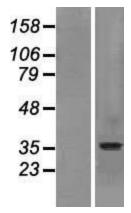
Western blot validation of overexpression lysate (Cat# LY424708) using anti-DDK antibody (Cat# [TA50011-100]). Left: Cell lysates from untransfected HEK293T cells; Right: Cell lysates from HEK293T cells transfected with [RC221202] using transfection reagent MegaTran 2.0 (Cat# [TT210002]).
