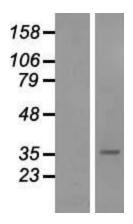
Western blot validation of overexpression lysate (Cat# LY418953) using anti-DDK antibody (Cat# [TA50011-100]). Left: Cell lysates from untransfected HEK293T cells; Right: Cell lysates from HEK293T cells transfected with [RC208391] using transfection reagent MegaTran 2.0 (Cat# [TT210002]).
