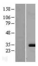
Western blot validation of overexpression lysate (Cat# LY418048) using anti-DDK antibody (Cat# [TA50011-100]). Left: Cell lysates from untransfected HEK293T cells; Right: Cell lysates from HEK293T cells transfected with [RC223662] using transfection reagent MegaTran 2.0 (Cat# [TT210002]).
