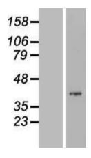
Western blot validation of overexpression lysate (Cat# LY413480) using anti-DDK antibody (Cat# [TA50011-100]). Left: Cell lysates from untransfected HEK293T cells; Right: Cell lysates from HEK293T cells transfected with [RC203877] using transfection reagent MegaTran 2.0 (Cat# [TT210002]).
