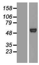
Western blot validation of overexpression lysate (Cat# LY409886) using anti-DDK antibody (Cat# [TA50011-100]). Left: Cell lysates from untransfected HEK293T cells; Right: Cell lysates from HEK293T cells transfected with [RC216088] using transfection reagent MegaTran 2.0 (Cat# [TT210002]).
