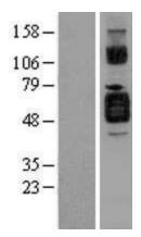
Western blot validation of overexpression lysate (Cat# LY401469) using anti-DDK antibody (Cat# [TA50011-100]). Left: Cell lysates from untransfected HEK293T cells; Right: Cell lysates from HEK293T cells transfected with [RC221860] using transfection reagent MegaTran 2.0 (Cat# [TT210002]).
