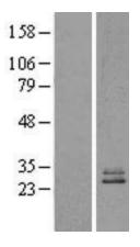
Western blot validation of overexpression lysate (Cat# LY401443) using anti-DDK antibody (Cat# [TA50011-100]). Left: Cell lysates from untransfected HEK293T cells; Right: Cell lysates from HEK293T cells transfected with [RC200567] using transfection reagent MegaTran 2.0 (Cat# [TT210002]).
