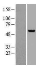
Western blot validation of overexpression lysate (Cat# LY400032) using anti-DDK antibody (Cat# [TA50011-100]). Left: Cell lysates from untransfected HEK293T cells; Right: Cell lysates from HEK293T cells transfected with [RC204074] using transfection reagent MegaTran 2.0 (Cat# [TT210002]).
