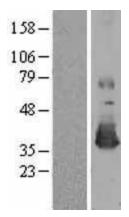
Western blot validation of overexpression lysate (Cat# [LY415828]) using anti-DDK antibody (Cat# [TA50011-100]). Left: Cell lysates from untransfected HEK293T cells; Right: Cell lysates from HEK293T cells transfected with [RC208916] using transfection reagent MegaTran 2.0 (Cat# [TT210002]).
