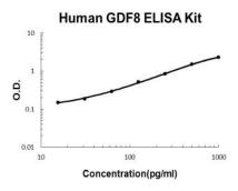
A standard curve is provided for demonstration only. A standard curve should be generated for each set of samples assayed.
