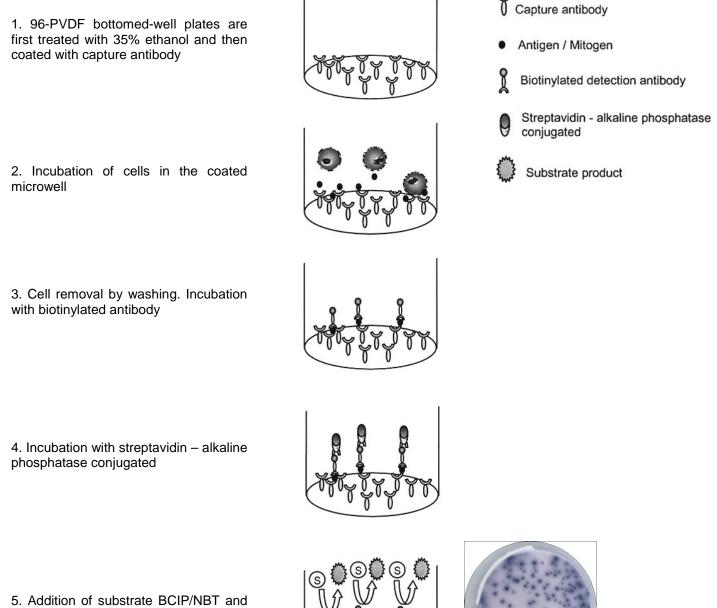
5. Addition of substrate BCIP/NBT and monitoring of spot formation.
