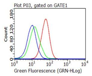
Flow cytometric analysis of living Raji cells, using anti-CD137L antibody ([TA813213], Red), compared to an isotype control (green), and a PBS control (blue) (1:100).
