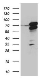
HEK293T cells were transfected with the pCMV6-ENTRY control (Left lane) or pCMV6-ENTRY RACGAP1 ([RC226045], Right lane) cDNA for 48 hrs and lysed. Equivalent amounts of cell lysates (5 ug per lane) were separated by SDS-PAGE and immunoblotted with anti-RACGAP1 (1:2000). Positive lysates [LY426645] (100ug) and [LC426645] (20ug) can be purchased separately from OriGene.
