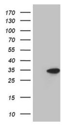
HEK293T cells were transfected with the pCMV6-ENTRY control (Left lane) or pCMV6-ENTRY IL24 ([RC216502], Right lane) cDNA for 48 hrs and lysed. Equivalent amounts of cell lysates (5 ug per lane) were separated by SDS-PAGE and immunoblotted with anti-IL24 (1:500). Positive lysates [LY416383] (100ug) and [LC416383] (20ug) can be purchased separately from OriGene.
