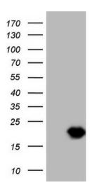
HEK293T cells were transfected with the pCMV6-ENTRY control (Left lane) or pCMV6-ENTRY TCAP ([RC203158], Right lane) cDNA for 48 hrs and lysed. Equivalent amounts of cell lysates (5 ug per lane) were separated by SDS-PAGE and immunoblotted with anti-TCAP (1:2000). Positive lysates [LY401215] (100ug) and [LC401215] (20ug) can be purchased separately from OriGene.
