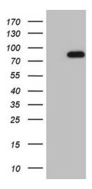
HEK293T cells were transfected with the pCMV6-ENTRY control (Left lane) or pCMV6-ENTRY HSF2 ([RC210751], Right lane) cDNA for 48 hrs and lysed. Equivalent amounts of cell lysates (5 ug per lane) were separated by SDS-PAGE and immunoblotted with anti-HSF2. Positive lysates [LY401434] (100ug) and [LC401434] (20ug) can be purchased separately from OriGene.
