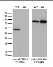
Equivalent amounts of cell lysates (10 ug per lane) of wild-type HeLa cells (WT, Cat# LC810HELA) and ALDH3A2-Knockout HeLa cells (KO, Cat# [LC832790]) were separated by SDS-PAGE and immunoblotted with anti-ALDH3A2 monoclonal antibody [TA503143] (1:500`). Then the blotted membrane was stripped and reprobed with anti-HSP90 antibody as a loading control.
