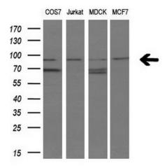
Western blot analysis of extracts (10ug) from 4 different cell lines by using anti-FGFR2 monoclonal antibody at 1:200 dilution.
