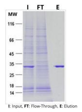
Demonstration of the purification process from beginning to end. Input lysate containing the impure protein. The flow-through indicating the desired protein has bound to the resin. Finally, the washed and eluted protein, exhibiting the high degree of purity at the end of the process.
