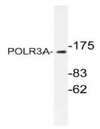
Western blot (WB) analysis of POLR3A antibody (Cat.-No.: AP21068PU-N) in extracts from HUVEC cells.
