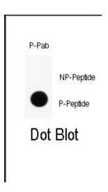
Dot blot analysis of anti-Phospho-ENT1 (Slc29a1)-pS254 Antibody on nitrocellulose membrane. 50ng of Phospho-peptide or Non Phospho-peptide per dot were adsorbed. Antibody working concentrations are 0.5ug per ml.
