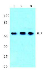
Western blot (WB) analysis of FLIP antibody at 1/500 dilution Lane 1:HEK293T cell lysate Lane 2:sp2/0 cell lysate Lane 3:PC12 cell lysate
