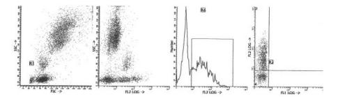
Representative Data Anti-CD38, clone T16, was analyzed by flow cytometry using a blood sample from a healthy donor. The cytogram shows direct staining with 10  $\mu$ l anti-CD38 R-PE per 100  $\mu$ l whole blood.
