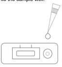
Immediately pipette 80µL p24 Running buffer into the sample well.
