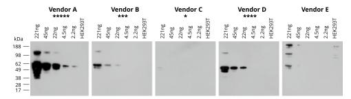
Five commercial antibodies against human P53 were evaluated in Western blot experiments with P53 over-expression cell lysate. P53 protein level in cell lysate was pre-determined using a purified GST-Myc-DDK standard. Lysate was serially diluted before SDS-PAGE and immunoblotting. Antibody quality and star rating is based on P53 protein detection level.
